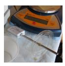
4. The small container with "food" was gently lifted off of the styrofoam cup, and the CuSO₄ and then Al were added. The small container was quickly placed back on top of the styrofoam cup, and the "Start" button on the computer was clicked to collect temperature data every 30 seconds until the temperature reached a maximum and began to decrease.
