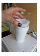
3. A wireless temperature probe connected to a computer was placed through the lid of the small container. A rubber band was used to set the position of the temperature probe, so the tip sat in the center of the water when the lid and temperature probe were placed on the small container.
