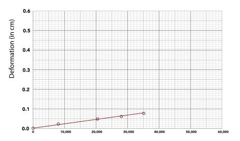
On each graph, the last point on the straight line is the **elastic limit.** This was the furthest amount the object could be deformed and still return to its original shape when the force on it was removed. Which material has a higher elastic limit, aluminum or steel?\_\_\_\_\_
